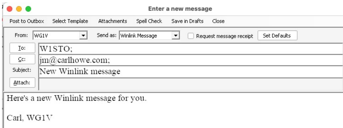
Figure 4: Figure 4: Winlink addresses can include Winlink user callsigns and standard email addresses separated by semicolons.
